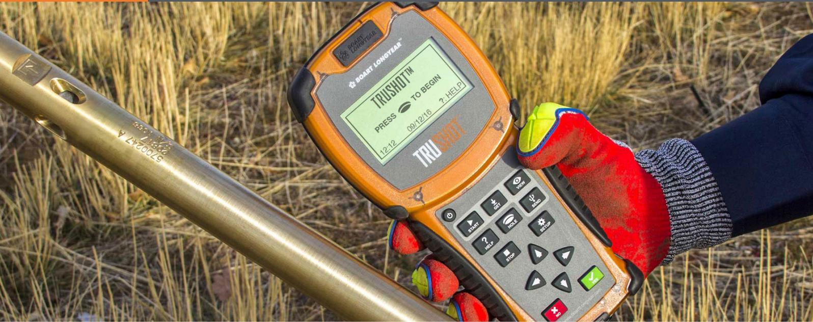
TruShot™ is an accurate magnetic survey tool optimized for driller deployment. Made for durability, precision and simplicity, drillers can capture high-quality 3D hole path data with confidence.
